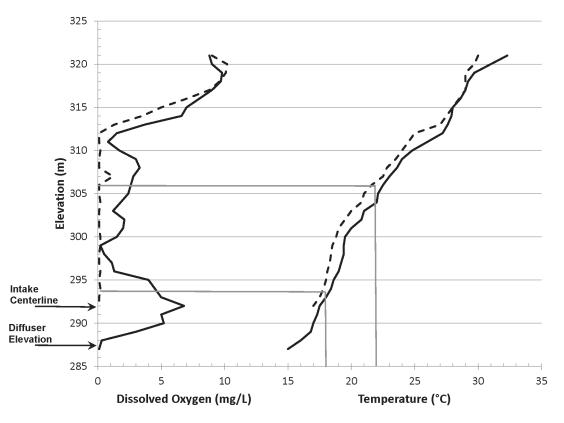
FIGURE 1. Dissolved oxygen and temperature profiles in Cherokee Reservoir, Tennessee, 14 August 1995, upstream (dashed lines) and downstream (solid lines) of oxygen diffusers (Mobley 1997). Elevations of the hydropower water intake and the oxygen diffuser are indicated. Gray lines indicate approximate depth of the estimated optimal temperature range for adult striped bass.
