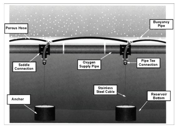
FIGURE 2. Schematic of diffuser system components.
